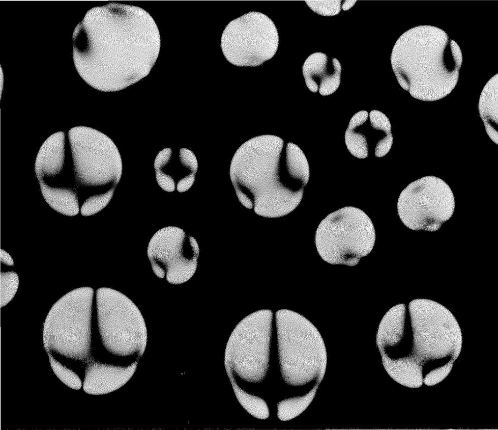
*These are droplets of the liquid crystal MBBA, formed in the process of cooling from a liquid phase. Viewed in polarized light, the liquid is black while the droplets show the birefringence characteristics of crystal structure.*
