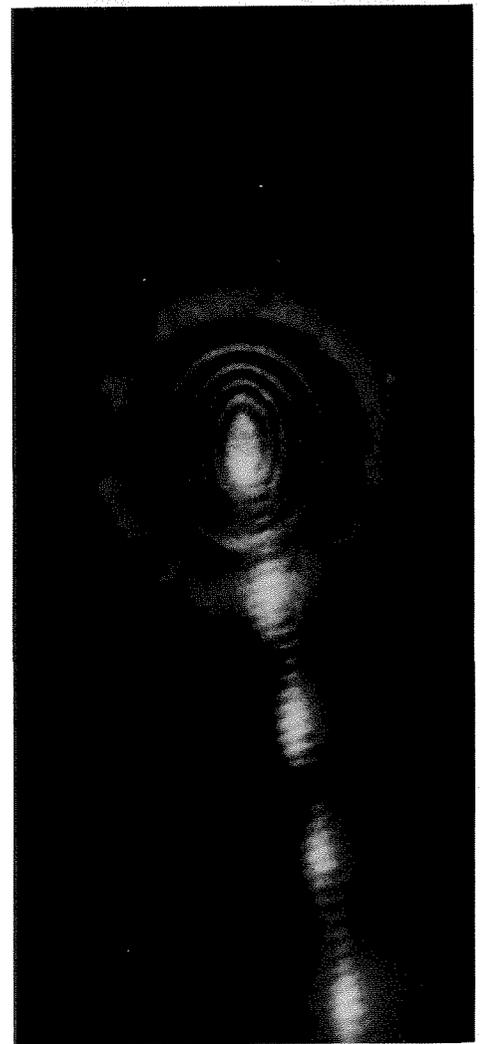
*This nematic liquid crystal (seen in polarized light) is deformed by the very intense visible light of a laser.*
