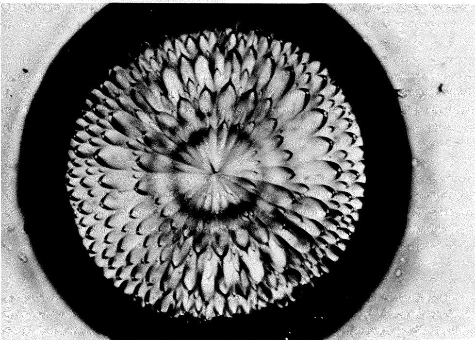
*This droplet of the most highly structured class of liquid crystal, seen in polarized light, displays a pattern of conic sections characteristic of the particular compound.*
