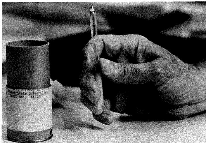
*The turbid material in this tube is a type of nematic "threadlike" liquid crystal known by the chemical shorthand MBBA, one of the few known to exist at room temperature. It was prepared by heating the constituents; if further heat is applied—such as a match flame—the MBBA would change to a clear liquid, recrystallizing when it cooled again.*
