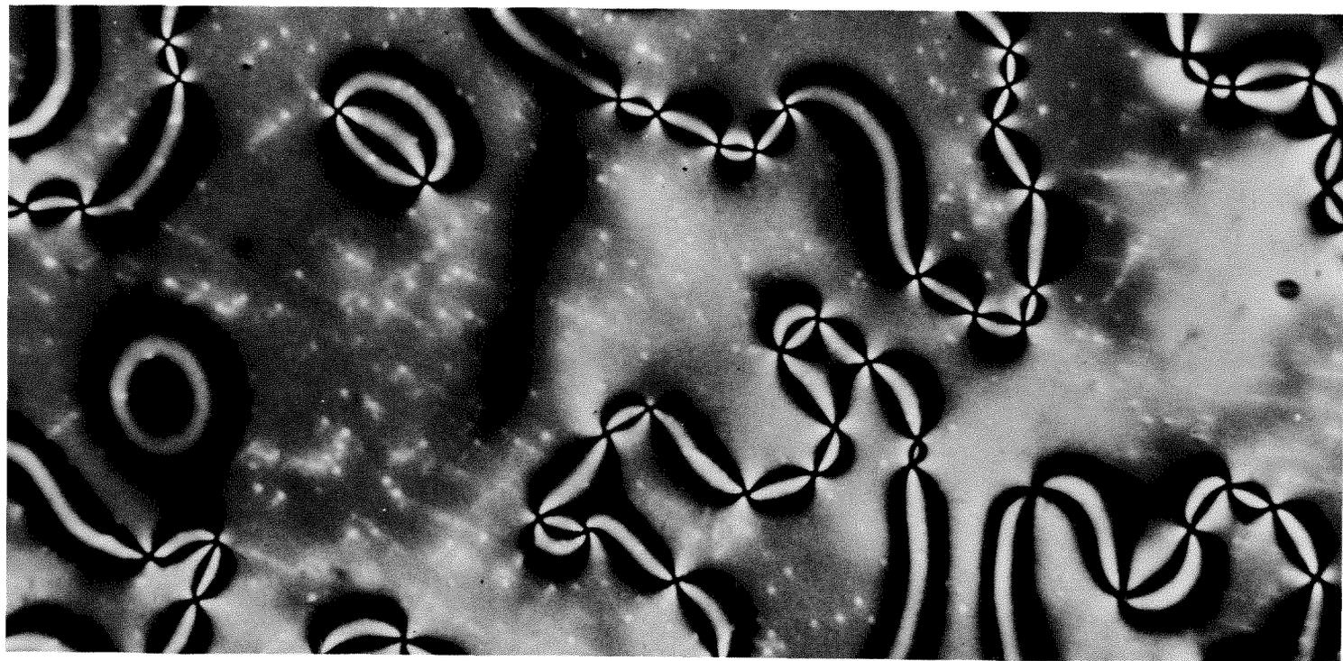
*All the molecules along any black curve are aligned in the same direction in this polarized light view of the nematic crystal MBBA.*
